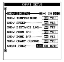
You can also turn the temperature, speedometer, distance log, zoom bar, zone alarm bar, and cursor on or off using this menu. See below for more information on these items.
